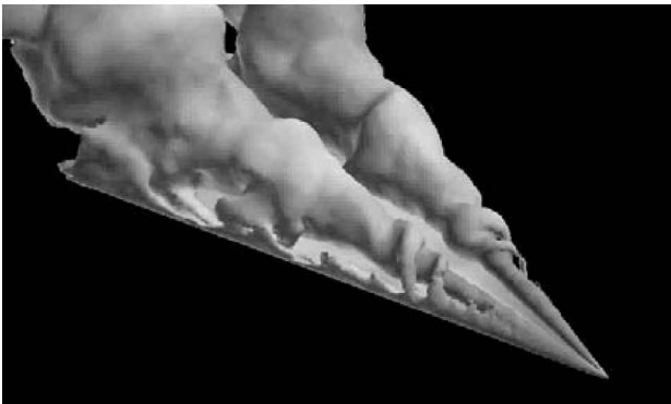
Fig. 10 Interaction between shear layer, secondary vortex, and primary vortex.
